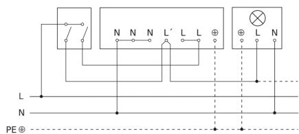
**Circuit diagram Connection via a changeover switch for continuous and automatic operation**
